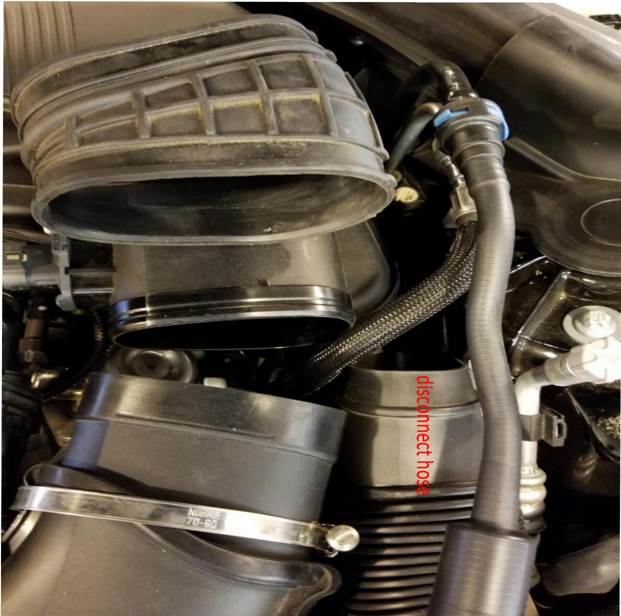
2. Disconnect the plastic hose located below the 2 clamps you just removed pictured above. There is a simple snap connection on the left and right side of the hose and should break loose with minimal force.
