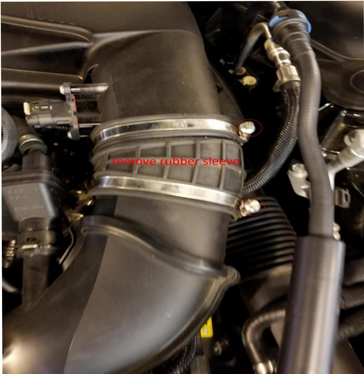
1. Remove the right-side rubber sleeve pictured above. This will allow you to disconnect the plastic hose below it, allowing you to more easily reach the driver side TMAP connection.
